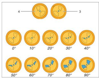
Water flow with opening angle 0° - 90°
