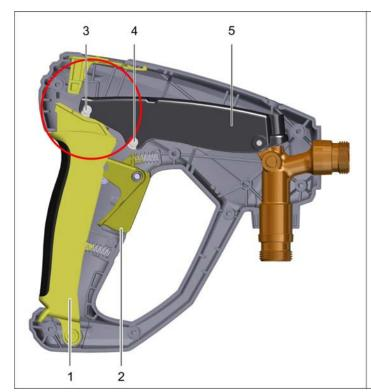
End position, gun opened Safety lever and trigger actuated.
